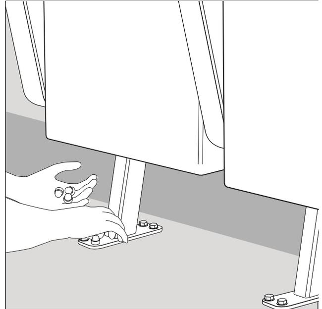
**Step 11:** Add supplied bolt caps to each bolt on the foot plate.
