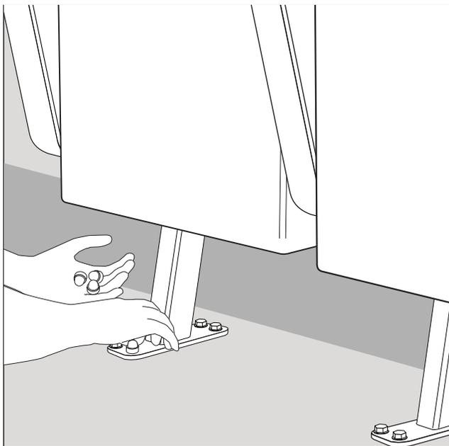
**Step 17:** Add supplied bolt caps to each bolt on the foot plate.
